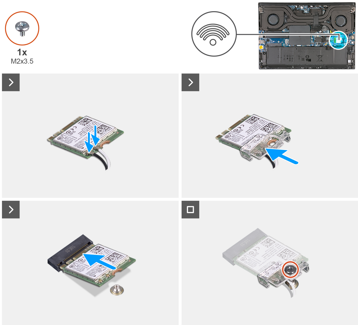
Figure 18. Installing the wireless card
