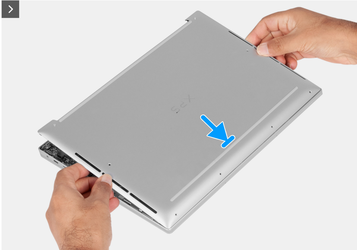
Figure 17. Installing the base cover
