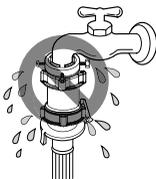
**2** If the tap is too large to fit the adapter, remove the guide plate.
