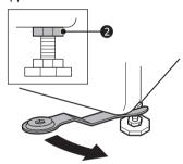
4 Check if all lock nuts at the bottom of the appliance are secured properly.
