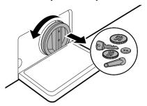
5 Clean the pump filter and opening with a brush.
