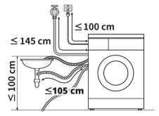
If the drain hose is too long, do not force it back into the appliance. This will cause abnormal noise.
