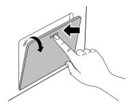
3 Remove the drain plug from the drain tube first, and then drain the water.
