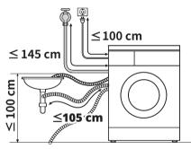
If the drain hose is too long, do not force it back into the appliance. This will cause abnormal noise.
