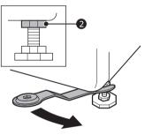
4 Check if all lock nuts at the bottom of the appliance are secured properly.
