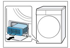
Ensure that the heat exchanger is inserted with its handle pointing downwards.
