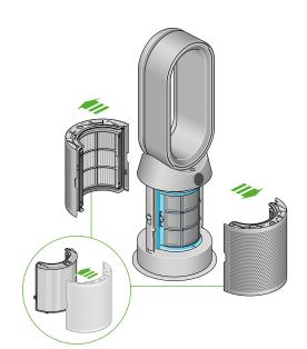
The air purifier fan heater with the filter covers open showing a HEPA plus carbon filter located in the filter covers and a catalytic filter. Arrows demonstrate that the catalytic filter is fitted directly to the base of the machine and the filter covers will need to be assembled onto the base of the machine.
