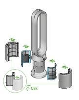
The air purifier fan with the filter covers open showing a 2 in 1 HEPA+ Carbon filter located in the filter covers and a catalytic filter. Arrows demonstrate that the catalytic filter is fitted directly to the base of the machine and the filter covers will need to be assembled onto the base of the machine.
