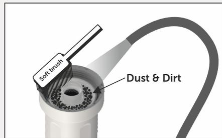
2. Clean the strainer mesh by soft brush and Water jet
