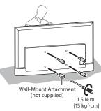
3 Attach the Wall-Mount Bracket (not supplied) using the screws (not supplied).
