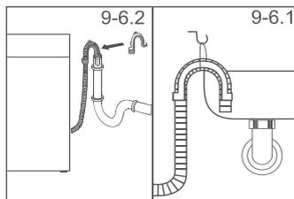
9.6.2 Drain hose to waste water connection
