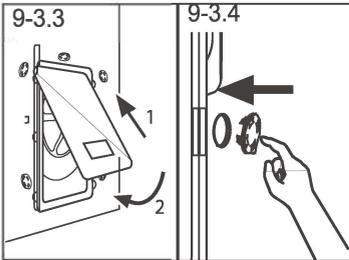
3. Replace back cover by inserting it in the two gaps its convexity is facing out (Fig. 9-3.3).
