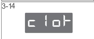
The display shows (Fig. 3-14) if a button will be pressed that means the child lock is activated. The change is not running.
