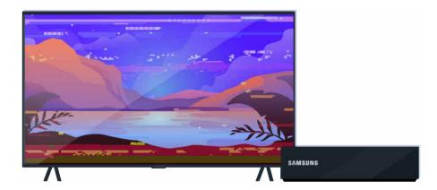
Check the antenna and input cable connections.
