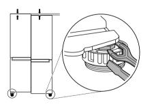
2 Open both doors and check to make sure that they close easily. If the doors do not close easily, tilt the refrigerator slightly more to the rear by turning both levelling legs to the left. It may take several more turns, and be sure to turn both levelling legs the same amount.
