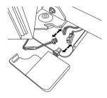
3 Remove the two hinge bolts.
