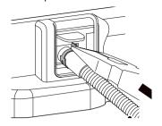
3 Screw in the band to secure the drain hose of the dryer onto the stacking bracket.
