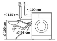
If the drain hose is too long, do not force it back into the appliance. This will cause abnormal noise.
