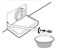
4 Unscrew the drain pump filter slowly to drain the remaining water and then proceed to remove any debris or objects from the filter.
