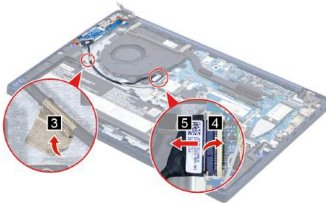
Figure 33. Peel off the tape and disconnect the USB board cable
