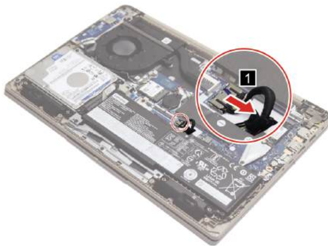
Figure 16. Disconnect the battery pack cable
