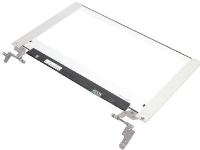
Figure 68. Remove the LCD assembly
