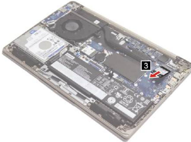
Figure 19. Remove the solid-state drive
