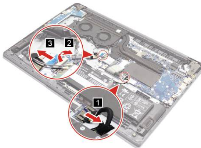
Figure 35. Disconnect the battery pack and the USB board cable
