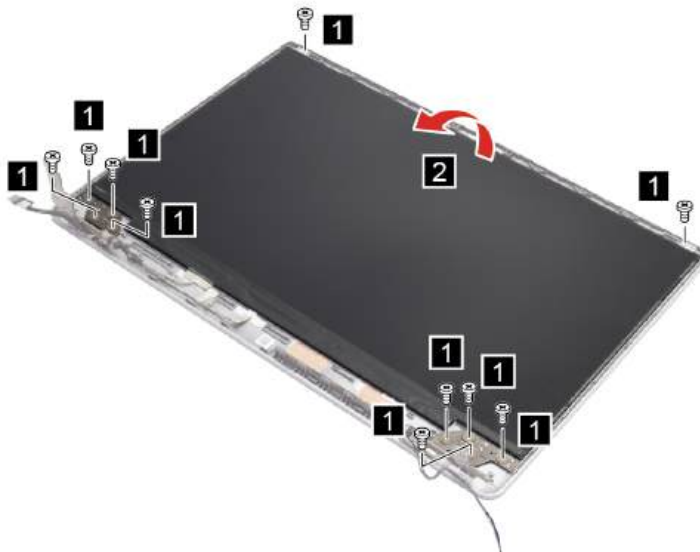
Figure 66. Lift the LCD assembly
