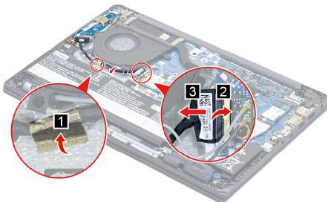
Figure 30. Disconnect the USB board cable from the system board
