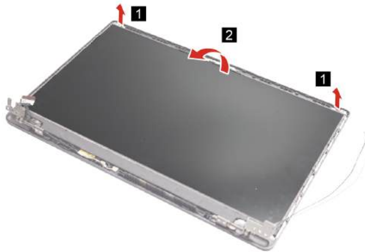
Figure 64. Lift the LCD panel
