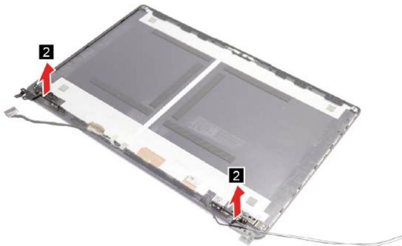
Figure 63. Remove the two hinges
