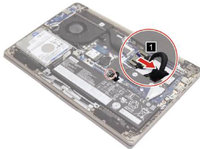
Figure 39. Disconnect the battery pack cable
