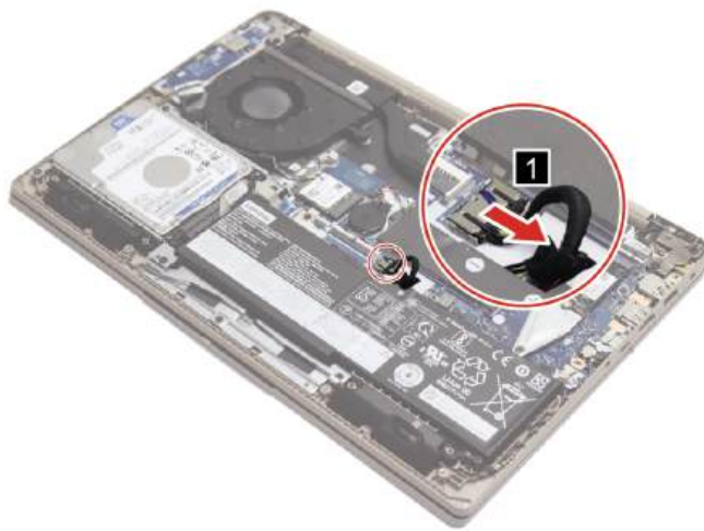
Figure 10. Disconnect the battery pack cable
