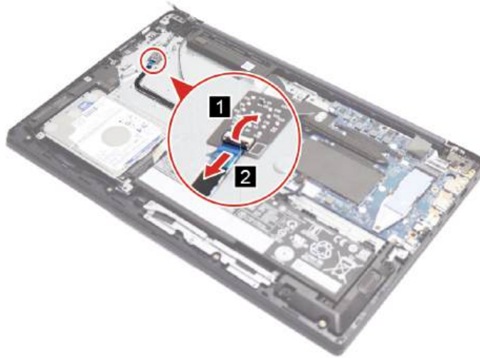
Figure 41. Disconnect the fingerprint reader cable
