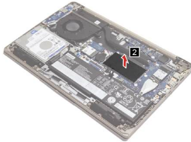
Figure 8. Remove the memory module shielding
