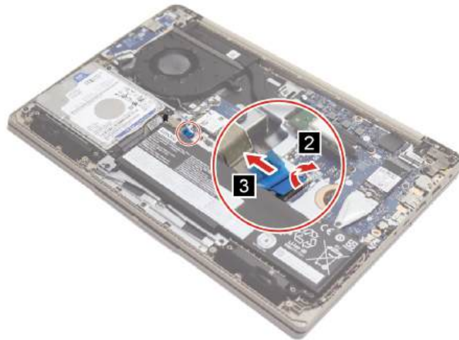
Figure 11. Disconnect the storage drive cable
