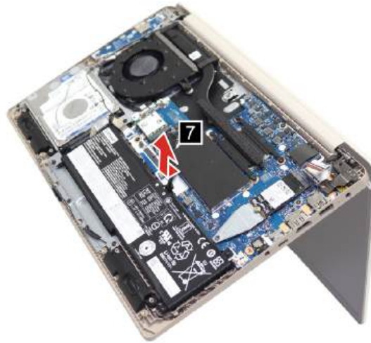
Figure 57. Remove the upper case assembly
