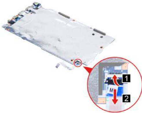
Figure 54. Remove the touchpad cable
