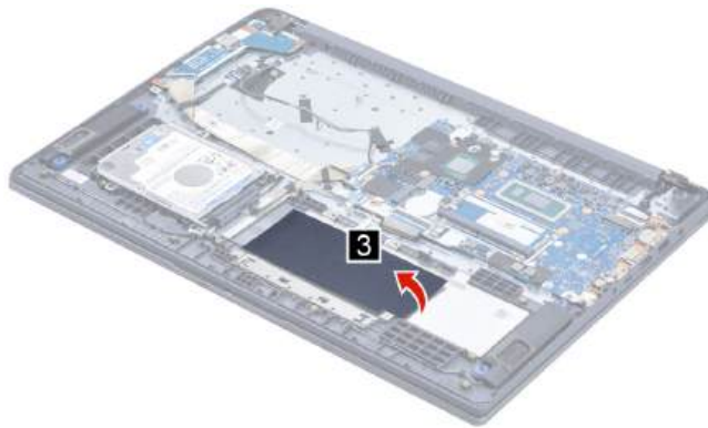
Figure 51. Peel off the touchpad tape
