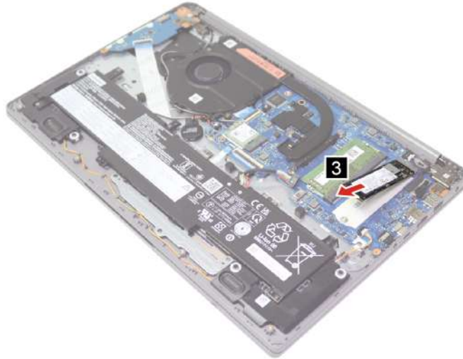
Figure 14. Remove the 2280 solid-state drive
