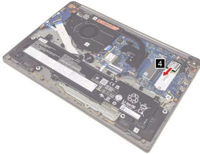
Figure 12. Remove the 2242 solid-state drive
