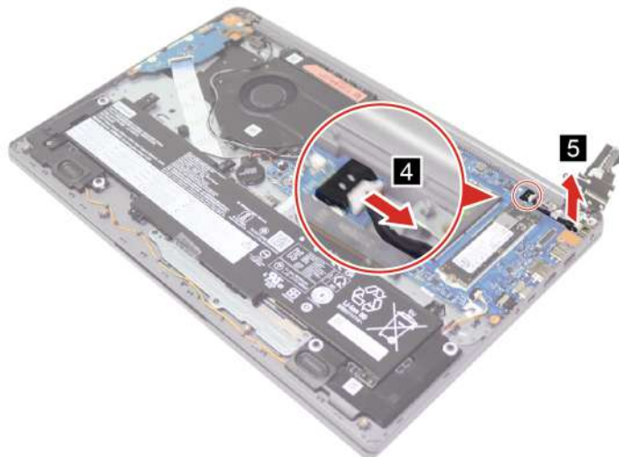
Figure 25. Disconnect and remove the DC-in cable
