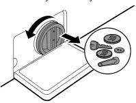
After cleaning the drain pump filter, carefully reinsert the filter and screw the drain cap back in clockwise carefully to avoid cross threading
