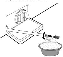
Unscrew the drain pump filter slowly to drain the remaining water and then proceed to remove any debris or objects from the filter.
