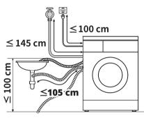
If the drain hose is too long, do not force it back into the appliance. This will cause abnormal noise.
