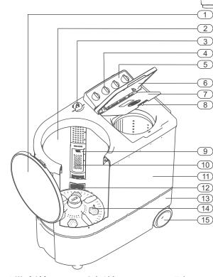
1. Wash Lid 6. Spin Lid 11.Tub 2. Wash Tub 7. Spin Inner Cover 12. Strainer 3. Water Selector 8. Spin Lid Handle 13. Under base 9. Water Level Indicator 14. Impeller 4. Knob 5. Decorative Panel 10. Cover Lint Filter 15. Big Wheel
