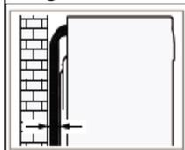
Do not trap the hoses and power cord between the wall and the appliance.
