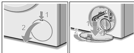
5. Take the drain hose out of the retainer. Remove the sealing cap, allow the water to flow out into a suitable container. Replace the sealing cap and place the drainage hose in the retainer.
