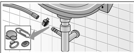
5. Reattach the drain hose and secure the connection using the hose clamp.
