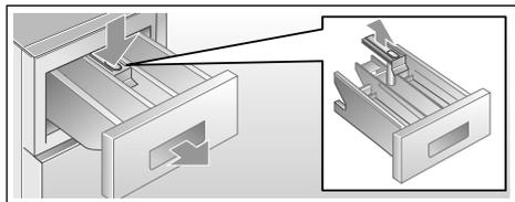
3. Clean the detergent dispenser tray and insert with water and a brush, and dry it. Clean the inside of the housing as well.
