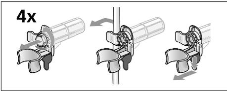
3. Fit the covers. Lock the covers firmly in place by applying pressure to the snap-in hooks.
