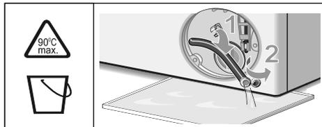
6. Carefully unscrew the pump cover, residual water may leak out. Clean the interior, pump cover thread and pump housing. The impeller in the detergent solution pump must be able to rotate. Refit the pump cover and screw it on tightly. The handle must be in a vertical position.
