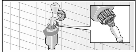
7. For standard and Aqua-Secure models, clean the filter on the rear of the appliance: Remove the hose from the rear of the appliance. Use pliers to remove the filter and then clean it.
