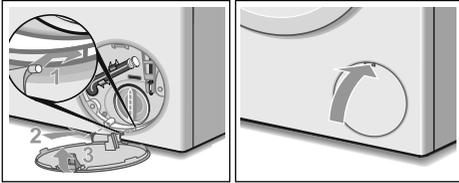
**Note:** To prevent unused detergent from flowing straight into the drain during the next wash, pour 1 litre of water (without detergent) into compartment **II** and start the **Spin/Drain//Spin/Empty** programme. Do the next wash as usual.
