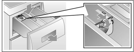
**Note:** Do not use the measuring aid for gel detergents and washing powder, or for programmes with prewash or when "👶" time is selected.
