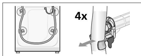
2. Unscrew and remove all four transport brace screws. Remove the sleeves. To do this, remove the mains cable from the holders.
