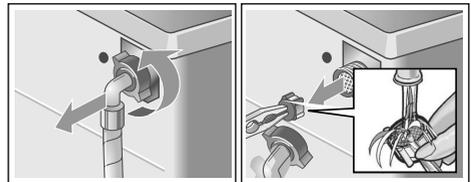
8. Insert the filter, connect the hose and check for leaks.
