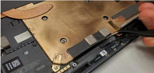
9. **Remove Thermal Module screws** – Use a 3IP (Torx-Plus) driver to remove the 14 screws securing the thermal module to the motherboard, designated with **3IP** and **3** in the device next to the screws. Use caution to not lose any screws in the enclosure during removal as they are not captive.
