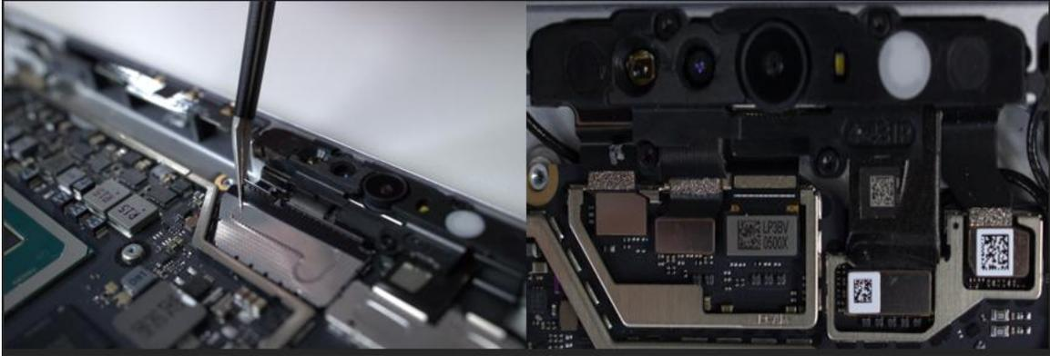
8. **Disconnect Camera FPCs** - Using the flat end of the Nylon spudger, gently disconnect 3 of the FPCs from the Motherboard.
