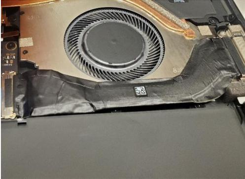
5. **Install the Display Module** – Install 2 new NFC foams. Reconnect the display FPC and install a new shield and shield tape on top. Align new PSA strips and install new speaker meshes on the display. Align the display on the bottom edge and press onto device. Use bonding frame tool to apply weight. Refer to the [Procedure – Installation \(Display Module\)](#) section for detailed instructions.
