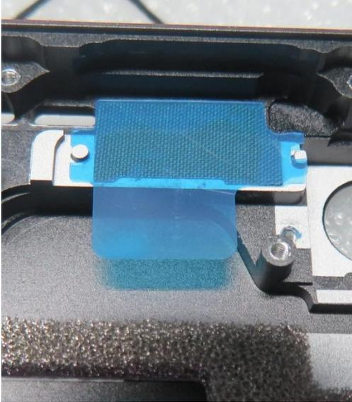
2. **Install the Front Facing Camera** – Remove the top liner from the PSA on the enclosure and camera. Using tweezers to handle the camera, install the camera by lining up the pin holes. Hold the camera down firmly for 10 seconds. Remove the camera cover when finished.
