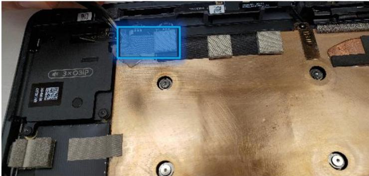
5. **Remove Buttons PCBA Screws** – Using a 3IP (Torx-Plus) driver, remove the 2 screws as shown in the image below (yellow circles) that are labelled with **3IP**. Once removed, lift the button board out of the device. If the button board is being reused, clean any residual tape from the board with IPA and cleaning swabs.
