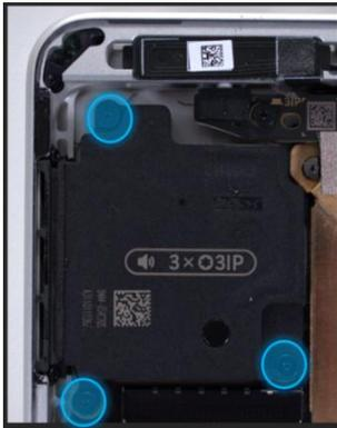
5. **Remove screws from right speaker** – Using a 3IP (Torx-plus) drive, remove the three marked screws from the right speaker and lift out of the enclosure. **DO NOT** remove the Graphite sheet – bend it as needed to access the speaker.
