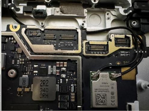
4. **Reconnect the Camera FPCs** – Using the flat end of a Nylon Spudger, align the 5 FPCs with their corresponding connector on the Motherboard. Press each down to complete the connection.
