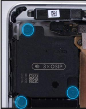
2. **Install the Right Speaker** – Place the right speaker into the enclosure making sure to align the screw holes on the speaker with the holes in the enclosure. Using a 3IP (Torx-plus) driver, install 3 screws from the bag labelled with **3IP** , turning each screw until finger tight then tighten each by an additional 1/8<sup>th</sup> turn (45-degrees). **DO NOT** remove the Graphite sheet – bend it as needed to access the speaker.
