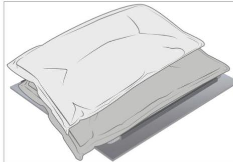
Shift second 9 kg steel shot bag to top edge of the device
