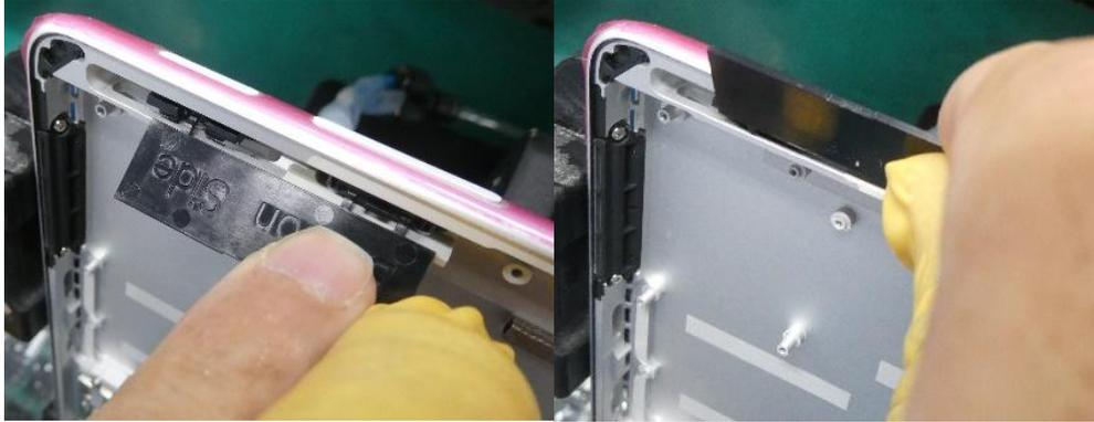
4. **Reinstall the NFC Module and Foams (if present)** – Install the PSA liner (13NL-5MU1B01) to the backside of the NFC module and press the NFC module back into the Enclosure. The PSA should sit behind the tab at the end and line up with the width of the module as shown below.
