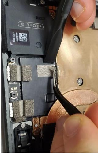
8. **Remove tapes and foams from the top edge** - Using a set of ESD-Safe Tweezers, remove the VC tape.
