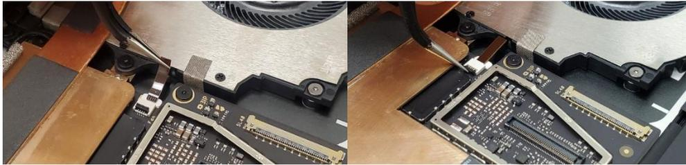
5. **Install Shielding Tape** – Using a set of ESD-Safe Tweezers, install the shielding tape beneath the left speaker as shown. Use the silver cutout on the shield as your starting point for the tape.
