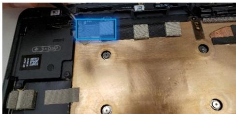
7. **Install the Display Module** - Install 2 new NFC foams. Reconnect the display FPC and install a new shield and shield tape on top. Align new PSA strips and install new speaker meshes on the display. Align the display on the bottom edge and press onto device. Use bonding frame tool to apply weight. Refer to the [Procedure – Installation \(Display Module\)](#) section for detailed instructions.
