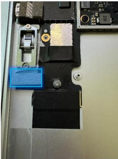
7. **Install the Thermal Module + Fan** – Apply new thermal pads to the thermal module or motherboard and place thermal module on top. Fasten 14 screws labelled with 03IP-1, 03IP-2, 03IP-3, 03IP-4 on the bags and reconnect the FPC to the motherboard. Apply a new VC tape to the thermal module. Refer to the [Procedure – Installation \(Thermal Module + Fan\)](#) section for detailed instructions.
