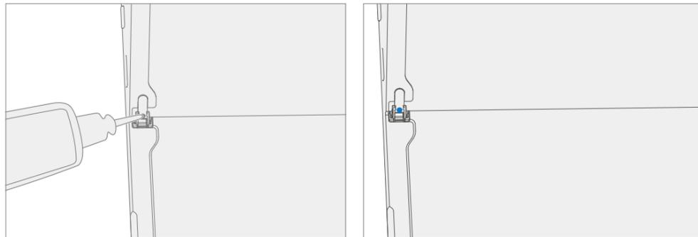
7. **Install hinge screws** – Use your finger to hold the back of the kickstand (shown below) while installing the screws (3IP Torx-Plus Driver) until they are fully seated in each hinge. Ensure the kickstand is properly aligned and seated in the hinges, then tighten each screw an additional ~quarter turn (~90 degrees). Be careful to only tighten the screws until snug to avoid stripping the kickstand threads. Ensure the screws do not fall into the hinge opening.
