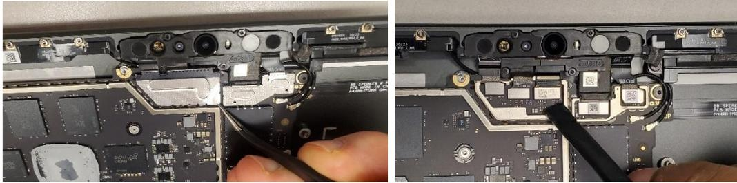
9. **Disconnect Wireless Coax Cables and Battery FPC** – Using the flat end of a plastic opening tool, disconnect the 2 coax cables from the motherboard. Using the flat end of a Nylon Spudger, disconnect the Battery FPC from the Motherboard.
