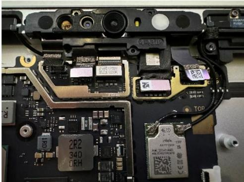
5. **Install RF tape** – Using your hands, or ESD-Safe Tweezers, place the tape near the bottom motherboard screw. Start by aligning the hole on the tape with the screw and carefully attaching the tape above and below that area. Use the etching on the enclosure to help guide alignment.
