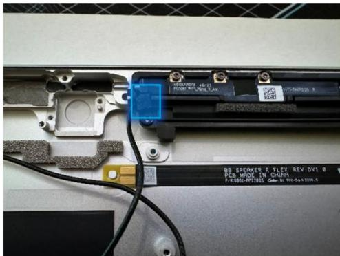
6. **Install the Rear Camera** – Install the rear camera with 2 screws (
