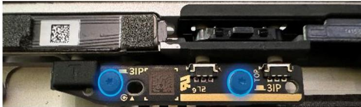
6. **Install tapes and foams** – Remove the liner from the new VC gasket (13NL-5LU0D11) and install it on the button PCB and thermal module. The top edge of the tape should align and cover the gold line on the PCB as shown.
