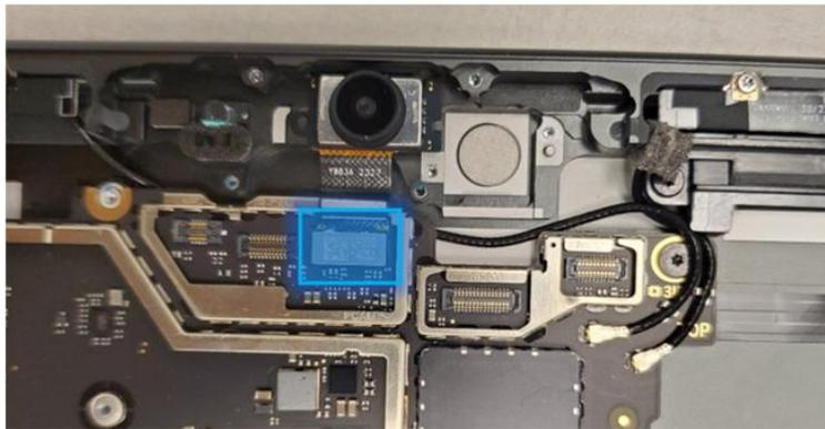
4. **Clean the camera** – Using a microfiber cloth, clean the lens before installing microphone module.
