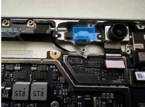
2. **Install the Microphone Module** – Place the new Microphone Module into the corresponding Enclosure gap ensuring the holes in the Microphone Module are in alignment with the Enclosure. Using a 3IP (Torx-plus) Driver, install the 4 screws from the bag labelled **3IP** until finger tight, then adjust each of them with an additional 1/8<sup>th</sup> turn (45-degrees) until secure. Fasten them in the order shown below.
