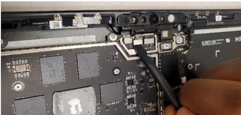
9. **Remove Microphone Module Screws** – Using a 3IP (Torx-plus) Driver, remove the 4 screws (
