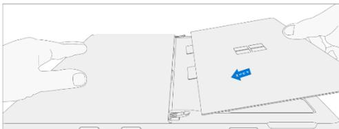
3. **Slot outer lip of each hinge into the Kickstand** – Using fingers on the underside of the kickstand and thumb on the topside, slightly rotate the kickstand on its axis as shown below. The kickstand should
