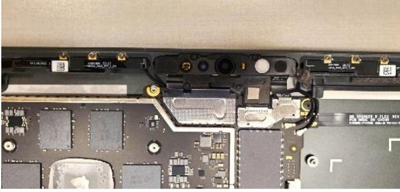
5. **Install the Thermal Module + Fan** – Apply new thermal pads to the thermal module or motherboard and place thermal module on top. Fasten 14 screws labelled with **03IP-1**, **03IP-2**, **03IP-3**, **03IP-4** on the bags and reconnect the FPC to the motherboard. Apply a new VC tape to the thermal module. Refer to the [Procedure – Installation \(Thermal Module + Fan\)](#) section for detailed instructions.
