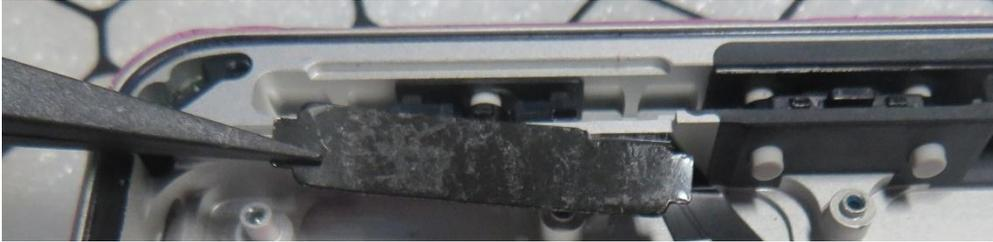
7. **Remove the Button clips** – Using a Nylon Spudger or a pair of ESD-Safe Tweezers, get under the edge of the button clip and leverage them up until the clip pops out. Remove both clips.
