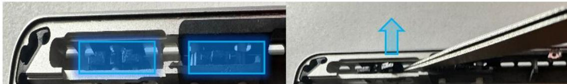
8. **Remove the Buttons** - Using a Nylon Spudger or a pair of tweezers, push on the button posts to remove the buttons from the enclosure.
