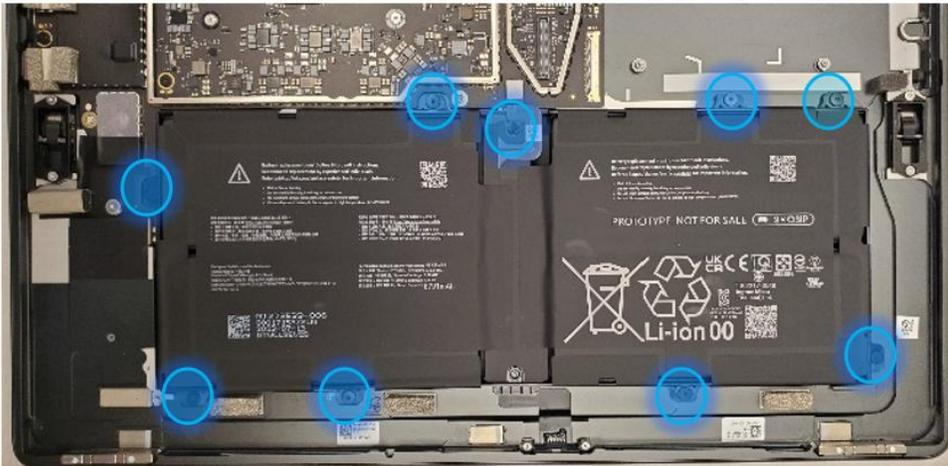
9. **Lift out the Battery** – Using two gloved hands, grab the battery by the frame at the points identified in the photo below and gently lift the battery out of the enclosure. Set battery on a clean, ESD-safe, flat surface. If reusing the original battery in the case of an enclosure replacement, lift and install the battery directly into the new enclosure after inspecting the device for any foreign objects and screws.
