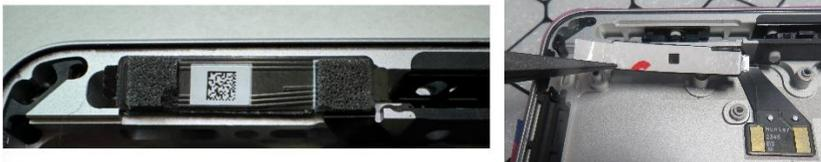
5. **Install the button PCB** – Insert the button PCB into the device, aligning the 2 screw holes with the screw bosses. Using a 3IP (Torx-plus) driver, install the two screws marked below with **3IP**, turning each screw until finger tight, then tighten each by an additional 1/8<sup>th</sup> turn (45-degrees).
