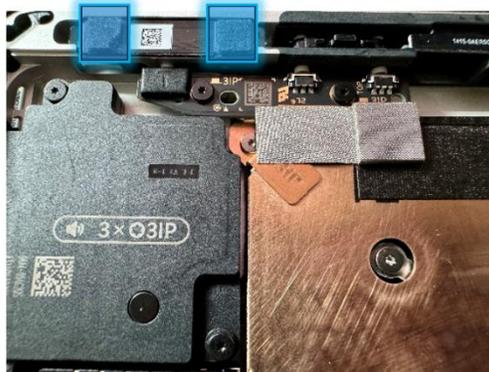
11. **Clean enclosure** - Using IPA and cleaning swabs, clean any residual adhesive from the enclosure edge. Ensure the area around the cameras (top edge) is clean and free of any dust or other contamination. Wipe the area around the camera with a lint-free cloth.
