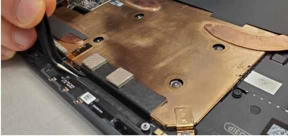
4. **Connect the Fan to the Motherboard** – Ensure the fan connector locking tab is up. Slide the Fan cable into the connector on the Motherboard. Press down on the locking tab to secure it. The FPC should slide in until the white lines are covered.
