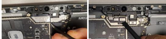
9. **Disconnect Wireless Coax Cables and Battery FPC** – Using the flat end of a plastic opening tool, disconnect the 2 coax cables from the motherboard. Using the flat end of a Nylon Spudger, disconnect the Battery FPC from the Motherboard.
