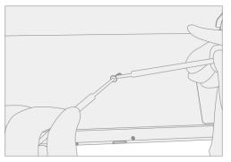
2. **Insert Foam Tabs** – With the hinges still at approximately 45-degrees, start to slide the new kickstand's foam tabs into the slots on the back of the device. Foam should slide in with minimal force – do not crumple the foam by using excess force. Do not slide the foam completely into the device – insert the foam tabs until approximately 3/4<sup>th</sup> of the foam tabs are inside the device.
