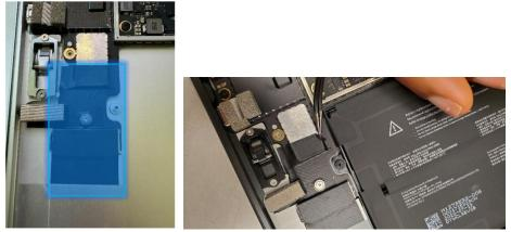
11. **Remove Motherboard screws –** Using a 3IP (Torx-plus) driver, remove 5 Motherboard screws labelled with #3IP .
