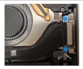
4. **Remove Surface Connect Port cable liner and install -** Remove the Surface Connect Port cable liner to expose the adhesive. Press down on the cable from left to right to glue the cable in place. Keep pressing along the cable to get rid of any bumps.
