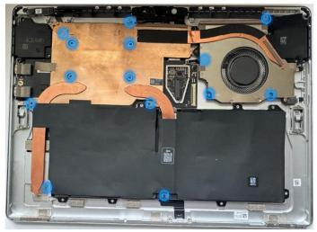
10. **Release the Thermal Module from the Motherboard –** Using the plastic opening tool, apply light pressure under each edge to slowly free the main plate from the thermal material underneath.
