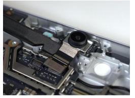
10. **Remove the Front Facing Camera –** Using the flat end of the plastic opening tool, position the tool under the FPC and lift to peel the camera off the enclosure.
