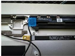
13. **Remove the Antenna Boards and Coax Cables –** Using a 3IP (Torx-plus) driver, remove the 6 screws holding in the Antenna Boards. The coax cables are attached to the boards, so do not separate them during removal. Lift out of the Enclosure and set aside for re-use.
