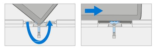
f. When you have reached the **bottom left corner**, rotate the device again in the Surface Debonding Tool track. Continue to push the device to the right through the Surface Debonding Tool track to cut through the left edge. Continue through the left speaker mesh area. The device may be pushed side-to-side along this edge to ensure separation between the screen and the device.
