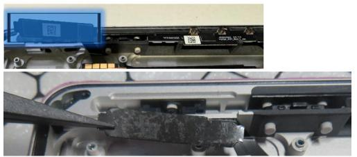
7. **Remove the Button clips –** Using a Nylon Spudger or a pair of ESD-Safe Tweezers, get under the edge of the button clip and leverage them up until the clip pops out. Remove both clips.
