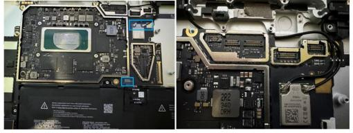
5. **Install the fan duct foam –** Using tweezers to hold the foam, carefully place the foam on top of the cable in the cutout shown below.
