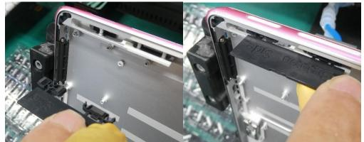
3. Remove the plastic tab – Bend the plastic tab front to back repeatedly until it breaks off from the clips.
