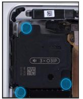
Install the Right Speaker – Place the right speaker into the enclosure making sure to align the screw holes on the speaker with the holes in the enclosure. Using a 3IP (Torx-plus) driver, install 3 screws from the bag labelled with **1**/8<sup>th</sup> , turning each screw until finger tight then tighten each by an additional 1/8<sup>th</sup> turn (45-degrees). DO NOT remove the Graphite sheet – bend it as needed to access the speaker.
