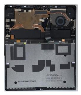
8. **Disconnect the display connector -** Remove the metallic tape from the shield lid using a pair of ESDsafe tweezers. Next, remove the shield lid on the display connector using the ESD-safe tweezers. Lift at the corners shown below and carefully free the shield lid. Disconnect the display connector by inserting the pointed edge of a Nylon Spudger under the left edge of the connector and peeling the connector off.
