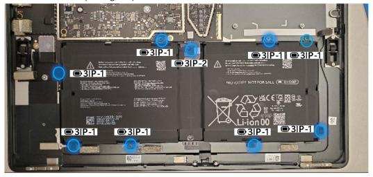
**Important:** Be careful not to overtighten screws. If the Battery frame is cracked or the battery is damaged in any way during installation, it cannot be used and must be replaced.
