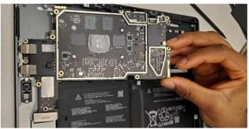
13. **Clean the enclosure –** Using IPA and cleaning swabs, clean any residual tape from the enclosure. If reusing the motherboard, clean the main chip and tape area with IPA and cleaning swabs.
