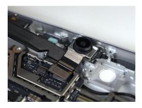
11. **Clean PSA –** Using tweezers or the Nylon spudger, remove the old PSA from the bucket and/or the camera. Clean the bucket area with IPA and cleaning swabs.
