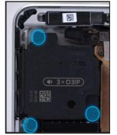
5. **Remove screws from right speaker –** Using a 3IP (Torx-plus) drive, remove the three marked screws from the right speaker and lift out of the enclosure. **DO NOT** remove the Graphite sheet – bend it as needed to access the speaker.
