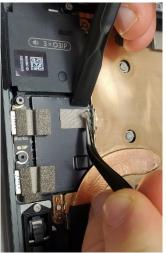
8. Remove tapes and foams from the top edge - Using a set of ESD-Safe Tweezers, remove the VC tape.
