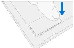
Procedure – Installation (Solid State Drive Door)
