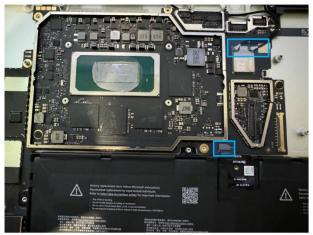
10. **Remove the RF foam and tape–** Using ESD-safe Tweezers, lift and remove the foam and shielding tape from the area shown. These will be replaced with new ones.
