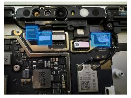
4. **Apply new Shields** – Using your fingers, assisted with the flat end of a Nylon Spudger, gently apply two new shields to cover the Camera FPCs. Using a finger, press on the edges to ensure a solid connection is made.
