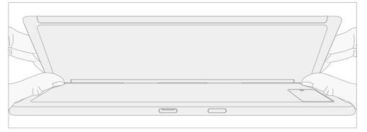
4. **Release the Kickstand threaded bosses** – Place your fingers on the underside of the kickstand, and your thumb on the topside. Slightly rotate the kickstand on its axis as shown below. The kickstand should rotate approximately 5 degrees to free the two threaded bosses of the kickstand from the recesses of the hinge.
