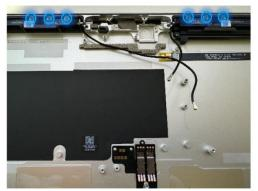
14. **Remove the fan duct Bracket –** Using a 3IP (Torx-plus) driver, remove the 1 screw securing the Bracket. Once removed, lift the Bracket out of the Enclosure and set aside for re-use.
