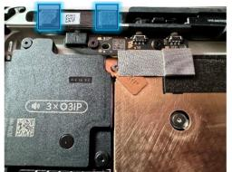
11. Clean enclosure - Using IPA and cleaning swabs, clean any residual adhesive from the enclosure edge. Ensure the area around the cameras (top edge) is clean and free of any dust or other contamination. Wipe the area around the camera with a lint-free cloth.
