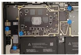
12. Lift the Motherboard out of the Enclosure – Using two hands, tilt the board to the left, and then pull the Motherboard out from the Enclosure. Ensure the USB connectors are free from the enclosure before fully removing the board to avoid damage. Do not damage the battery or cameras during disassembly.
