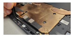
4. **Connect the Fan to the Motherboard –** Ensure the fan connector locking tab is up. Slide the Fan cable into the connector on the Motherboard. Press down on the locking tab to secure it. The FPC should slide in until the white lines are covered.
