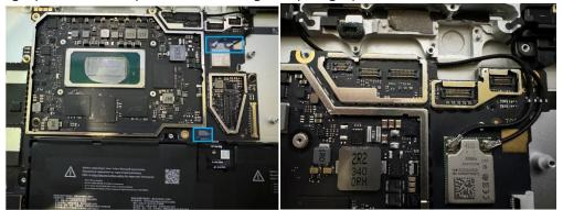
4. **Reconnect the Camera FPCs –** Using the flat end of a Nylon Spudger, align the 5 FPCs with their corresponding connector on the Motherboard. Press each down to complete the connection.
