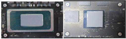
2. Install the Thermal Module – Align the thermal module and fan to the screw holes on the motherboard. Gently lower the Thermal Module into place. Fasten the screws in the order of the dash numbers, starting with the @3IP-1 screws and working your way to end with the @3IP-4 screws. The order for each screw is shown below. Note: The @3IP-4 screws around the main chip on the motherboard are installed in an "x" pattern.
