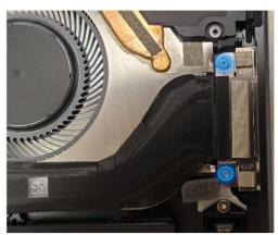
6. **Remove the Surface Connect Port cable** – Gently peel the Surface Connect Port up from the chassis from left to right. Clean any residual adhesive left behind on the thermal module with IPA and a cleaning swab. When reusing the Surface Connect, peel off the residual adhesive from the Surface Connect.
