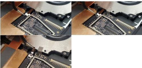
7. **Remove Shielding Tape –** Using a set of ESD-Safe Tweezers, remove the shielding tape beneath the left speaker as shown. Be careful not to remove the shield from underneath using a Nylon spudger to hold it down.
