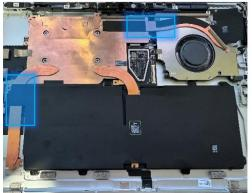
12. Clean any Thermal Interface Material from the Motherboard – Using a Nylon Spudger, scrap any remaining Thermal Interface Material from the Motherboard. Use IPA and Cleaning Swabs to clean any residual Thermal Interface Material.
