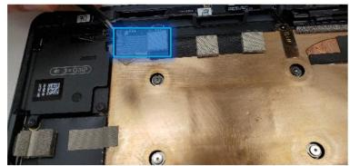
Remove Buttons PCBA Screws – Using a 3IP (Torx-Plus) driver, remove the 2 screws as shown in the image below (yellow circles) that are labelled with -3IP . Once removed, lift the button board out of the device. If the button board is being reused, clean any residual tape from the board with IPA and cleaning swabs.
