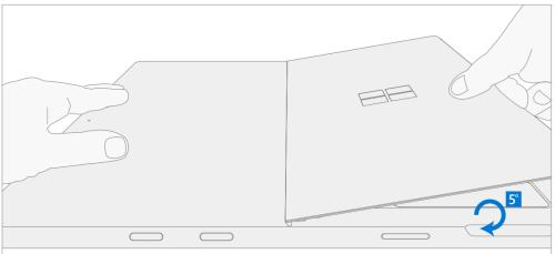
5. **Remove the Kickstand** – Using the palm of your hand, firmly hold the device from the center of the chassis. Simultaneously, grip the kickstand off-center between your thumb and index finger and firmly pull. Pull with a moderate amount of force until the foam inserts slide out of the device. If the kickstand is stuck, ensure the threaded bosses have not slipped back into the recesses on the hinge.
