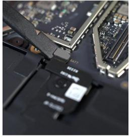
8. Remove the Battery Screws – Remove the 9 screws from the Battery frame using a 3IP (Torx-plus) driver.
