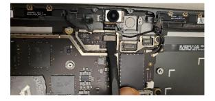
9. **Remove the Front Facing Camera (Re-use only) –** Install the camera cover (13NL-5LU1301) on the lens. Using the flat end of the plastic opening tool, position the tool under the right side of the FPC, and carefully lift to peel the camera off the enclosure.
