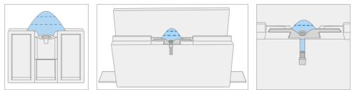
b. Clamp the debonding tool to the edge of your workbench using a Hand Clamp on each side as shown in the image below. Ensure the cut depth adjust can be accessed while the tool is clamped down. If it cannot be accessed, the clamps will have to be removed to access the bottom of the tool and then re-clamped after adjusting the height.
