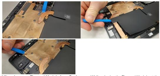
11. Lift and remove Thermal Module from Enclosure – While gripping the Thermal Module at the specific points shown below, slowly lift and twist clockwise to free it from the enclosure. Do not damage or wrinkle the Graphite sheets.
