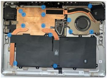
**Important:** The Thermal Module is very fragile. Take extra care not to bend or twist the Thermal Module + Fan assembly. If any part of the Thermal Module or its heat pipes are bent, then the whole module must be replaced.
