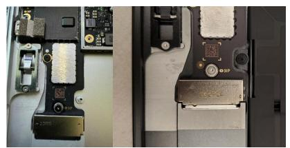
6. **Install RF Foam on the RF tape –** Place the Foam on top of the Shielding Tape. The top and left edges should align to the edges of the tape as shown.
