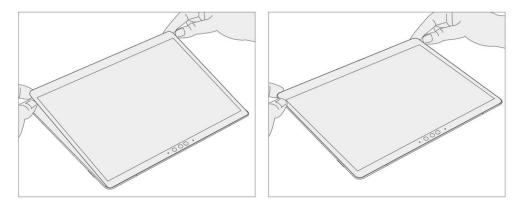
6. **Bond the adhesive –** Place the Surface Display Bonding Frame on the device, ensuring that the cutouts on the sides line up with the buttons. Place a foam pad over the bonding frame. Place 32 kg of weight on top of the foam pad and bonding frame. Leave weight in place for 2 minutes to ensure PSA activation.
