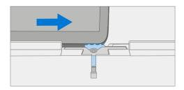
**CAUTION:** Do not insert the pick more than 2mm along the left, right, or bottom edges of the display. The pick depth should not exceed 8mm along the top edge of the display.
