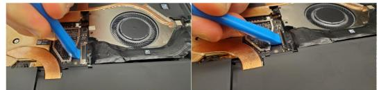
5. **Remove the Surface Connect Port screws –** Use a 3IP (Torx-plus) driver to remove both Surface Connect Port screws labelled with **43IP**.
