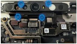
3. **Reconnect the Camera FPCs –** Using your fingers, or the flat end of a Nylon Spudger, reconnect the 3FPCs to the corresponding connectors on the Motherboard.
