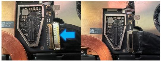
Install Surface Connect Port screws – Insert the port into the enclosure on the right with a toe-in. Use a 3IP (Torx-plus) driver to install 2 screws labelled 43IP until they are just snug and seated. Turn each screw another 45 degrees (1/8 turn) until fully fastened.
