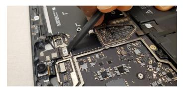
9. **Remove Rear Camera Screws –** Using a 3IP (Torx-plus) Driver, remove the 2 screws ( **O**3IP ) outlined in the photo below. Once removed, lift the Rear Camera out of the enclosure.
