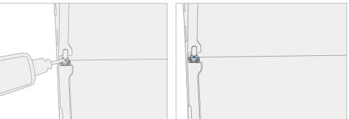
7. Install hinge screws – Use your finger to hold the back of the kickstand (shown below) while installing the screws (3IP Torx-Plus Driver) until they are fully seated in each hinge. Ensure the kickstand is properly aligned and seated in the hinges, then tighten each screw an additional ~quarter turn (~90 degrees). Be careful to only tighten the screws until snug to avoid stripping the kickstand threads. Ensure the screws do not fall into the hinge opening.
