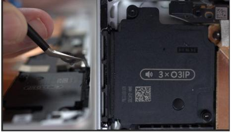
10. **Remove foams from the NFC** – Locate the NFC in the top-left corner of the device. Using the Nylon spudger, carefully remove 2 foams from the NFC. These will be replaced.
