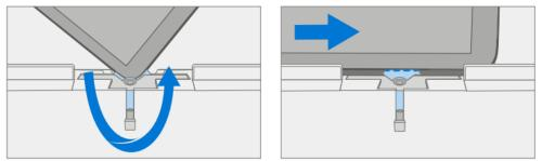
When you have reached the **top left corner**, rotate the device in the Surface Debonding Tool track. Push the device to the right through the Surface Debonding Tool track to cut through the top edge. It is normal to feel more resistance on the top edge compared to the other edges due to the cameras. Continue to carefully add force and push the device over the pick.
