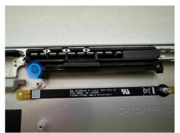
15. **Remove the Battery** – Remove 9 screws. Lift the battery from the original enclosure and install it directly into the new bucket. Lift the battery from the sides on the frame. Refer to the <u>Procedure – Removal</u> (<u>Battery</u>) section for detailed instructions.
