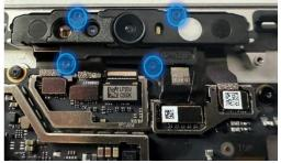
10. **Thermal Putty Cleanup –** Clean the light blue/green putty as shown with IPA and cleaning swabs until the area is free of any residual T-Putty.
