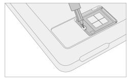
4. **Remove the Removable Solid-State Drive –** The rSSD should lift upwards to approximately 15-degrees after the screw is removed. Carefully grab the sides of the rSSD case and pull it out of the Motherboard socket at the same approximately 15-degree angle. A Nylon Spudger can be used to lift the rSSD up.
