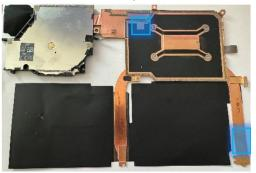
**b.** Apply the CPU pad (13NL-5LU0Q01) to the center of the main chip on the motherboard as shown below. Remove the plastic liner from all pads when ready to install the thermal module.
