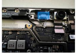
Install the Microphone Module – Place the new Microphone Module into the corresponding Enclosure gap ensuring the holes in the Microphone Module are in alignment with the Enclosure. Using a 3IP (Torxplus) Driver, install the 4 screws from the bag labelled **\$3IP** until finger tight, then adjust each of them with an additional 1/8<sup>th</sup> turn (45-degrees) until secure Fasten them in the order shown below.
