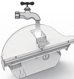
**3** Fill the dirty water tank with clean water. Close the cap and shake.
