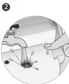
Press the lock button and clean the fan-coil outlet.
