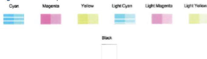
Figure 9-2 Example of color blocks with defects
