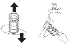
To replace the assembled filters, position the spray arm so the wider vee is toward the front. Fit the filters back into the filter holder and secure them by turning the inner filter clockwise until it clicks into place.
