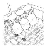
The left side row of tines can be folded down or the cup racks can be folded up out of the way for tall crockery items.
