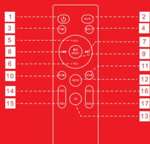
1. Power Button: Standby mode for Power ON/OFF.
