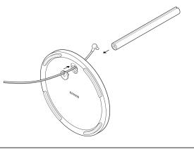
Fasten the base (with the washer) tothe stand pole using 1 black screw(included) and a Phillips-headscrewdriver. Make sure the cord canstill slide freely.
