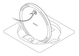
Position the washer with the alignment pins facing in. Then align the stand pole with the base, using the alignment pins to guide you.
