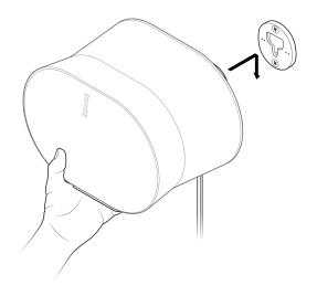
To adjust for optimal sound, unlock the speaker by rotating the collar on the mount 90° counterclockwise. Reposition the speaker, then rotate the collar 90° clockwise to lock.
