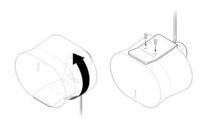
Align the mount with the bracket keyhole, slide the mount down, and lock it into place. Make sure the wall mount and speaker are securely seated before removing your hands from the speaker.
