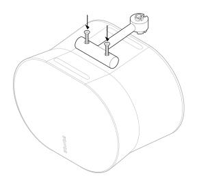
Attach the speaker platform to the stand pole using the other screw (included). Then plug the power cord into the speaker. You may need someone to hold the speaker for this step.
