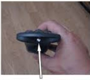
With a button pressed and held, the IR LED doesn't look any different.
