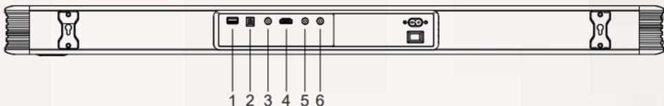
**1. USB IN:** Used to connect a flash drive for direct MP3/WAV playback (FAT32 format and 32GB max).
