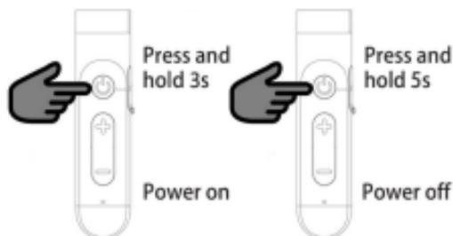
Power on:- Press and hold the multifunction (MFB) for 3s until the BLUE light flashes.
