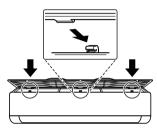
6 To make sure the filter is assembled properly, press down along the entire front length of the filter.
