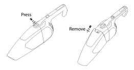
2. Clear the dust cup. A soft brush can be used to clean dust on filter.
