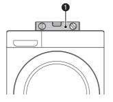
3 Secure the levelling feet with the lock nuts by turning anti-clockwise against the bottom of the appliance.
