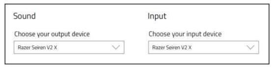
When set as the default output device, an audio output device (such as a headphone) must be connected to its 3.5 mm headphone port. This will allow you to listen to the audio output and recording at the same time.
