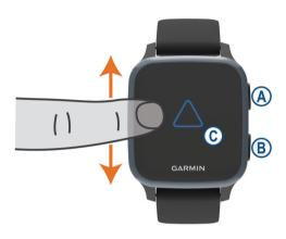
Action button: Press to turn on the device. Press to start and stop the activity timer.
