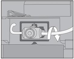
**Useful tip:** If necessary, turn the milk pipework towards the back at the connecting piece on the right-hand side.
