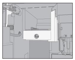
Remove the milk valve cover: press on the recessed grip to unlock the cover. On the top right-hand side of the cover, you will find a pin for swivelling the cover out.
