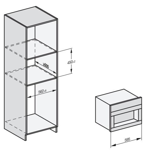
Combination with other Miele Built-in Appliances is possible. If the coffee machine is to be built in above another appliance, there must be a full-width, closed shelf between them. If the machine is to be combined with a suitable built-in dishware / food-warming drawer, no shelf is required in between.
