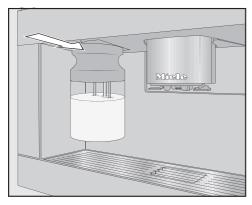
Push the milk container back into the coffee machine until it clicks into place.
