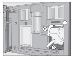
■ Pull the brew unit to the side ① first and then pull out to the front ②. Tilt the brew unit forward ③ while doing so.
