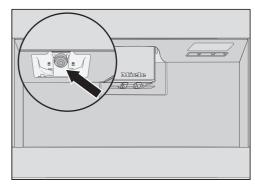
Clean the milk container holder on the coffee machine with a damp cloth.
