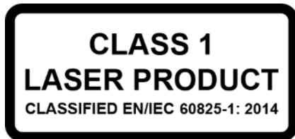
Figure 6. ToF sensor laser safety compliance mark
