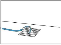
Secure the elbow to the gully.
