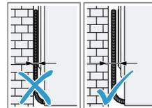
Do not trap the hoses and power cord between the wall and the appliance.
