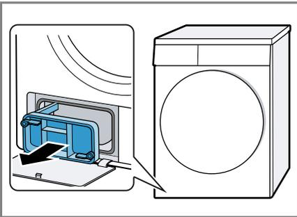
2. Clean the heat exchanger cover under running water and dry it.
