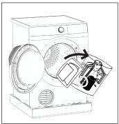
Put one of the polystyrene packaging elements on the floor behind the appliance. Carefully put down the appliance with the rear side on it.
