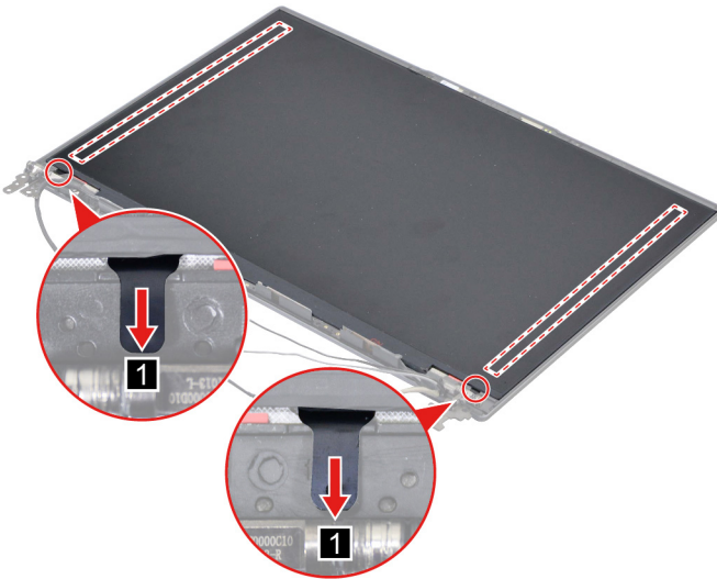
Figure 34. Remove the two pieces of removable tape with tweezers
