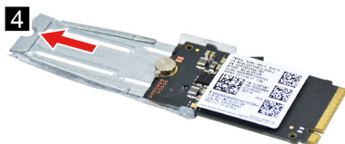
Figure 12. Remove the SSD bracket
