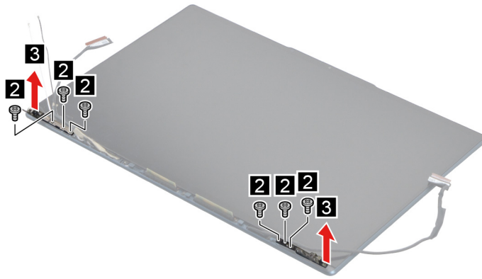
Figure 45. Remove six screws and remove the hinges
