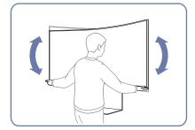
• Hold the bezel at both side edges and adjust the monitor angle until the screen becomes level. (Be careful not to directly hold the LCD display.)
