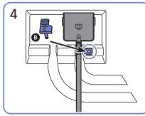
Insert the cable holder into the hole to fix the cables.
