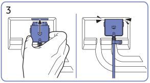
Connect the cables to the corresponding ports.
