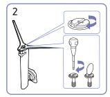
Tightly fasten the connecting screw at the bottom of the stand base.
