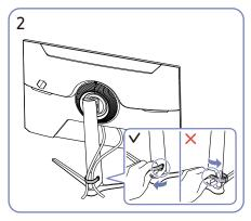
Pull the right side of the HOLDER-STAND CABLE to remove from the stand. The left side of the HOLDER-STAND CABLE can be damaged when pulled forcibly.
