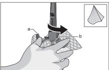
6. Put fibre- and brass-washer onto the axis. Put the assembly into the jar.
