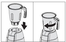
3. How to fit/remove active flow breaker Your Bosch TrueMixx Style Mixer Grinder has an active flow breaker which improves the quality of your wet grinding applications. To fit the active flow breaker, insert the active flow breaker in the groove on the inside surface of the big jar and slide it in until it fits properly. To remove it, gently press in the opposite direction till it disengages. Slide it out thereafter.
