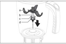
7. Put the plain washer and spring onto the axis from the underside and tighten the coupler by rotating it in an anti-clockwise direction.
