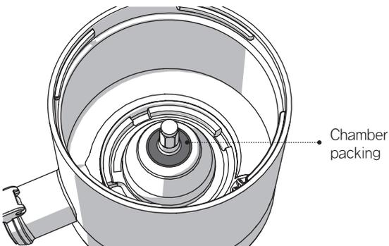
The chamber packing can't be disassembled.
