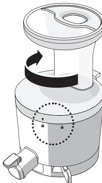
After [ Step 3 ], match [ ▼ ] of the hopper to [ 🔒 ] on top of the chamber in a straight line and turn it clockwise until it comes to [ 🔒 ].
