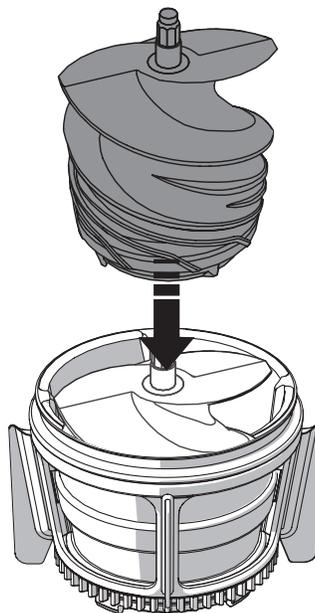
Assemble the screw into [STEP1].
