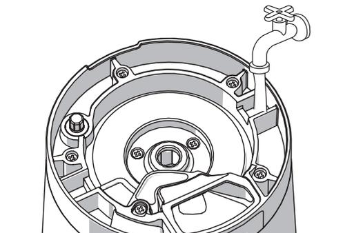
When you clean the chamber set, wash the residue inside and bottom of the chamber under running water.
