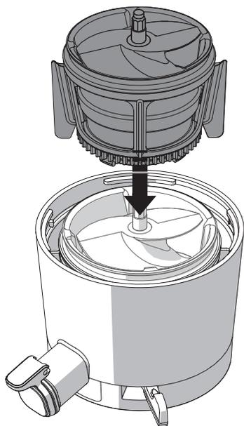
Place the assembly form [ Step 2 ] into the chamber and turn left and right until the bump on the bottom of the net falls into the groove inside the chamber.
