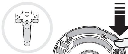
Push the intermediate gear from the bottom side of the chamber to remove the gear.
