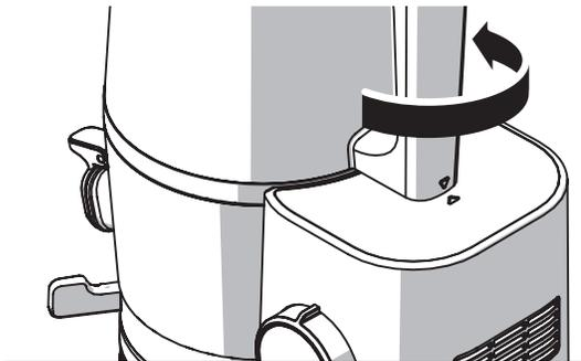
If the chamber is not easily separated from the hopper, separate the hopper, while the chamber is connected to the main body, and wash the hopper in running water.
