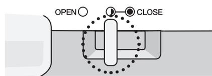
When extraction is almost finished, place the control lever into [ ◐ ] half-opened position.
