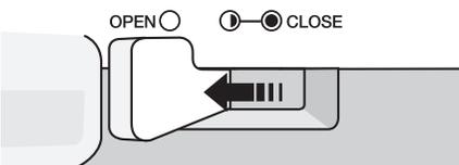
You cannot move the control lever to [ ○ OPEN ] position when the chamber is placed on the main body.
