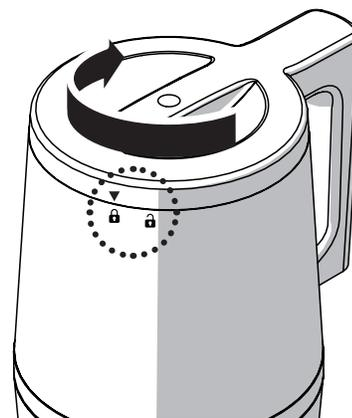
After [ Step 5 ], align [ ▼ ] on the lid with [ 🔒 ] on the upper side of the hopper in a straight line and turn it clockwise until the icon on the lid points [ 🔒 ].
