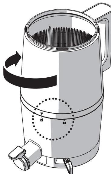
After [ Step 3 ], match [ ▼ ] of the hopper to [ 🔒 ] on top of the chamber in a straight line and turn it clockwise until it comes to [ 🔒 ].
