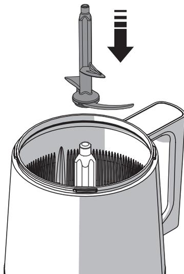
After [ Step 4 ], fit the mixing bar on the shaft of the screw.
