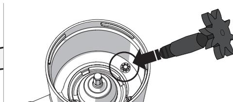
Place the intermediate gear after cleaning.
