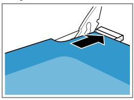
Push the pane into both openings on the underside. The smooth surface of the pane must face outwards.
