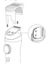
the length range of 0.5–10 mm and 10.5–20 mm. Choose the appropriate trimming comb according to your needs.
