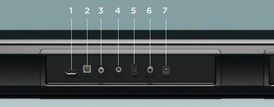
1.HDMI(ARC): Use to connect compatible devices using a HDMI cable (not provided).
