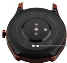
Connect the magnetic end of the charger here & the other end to an adapter/laptop
